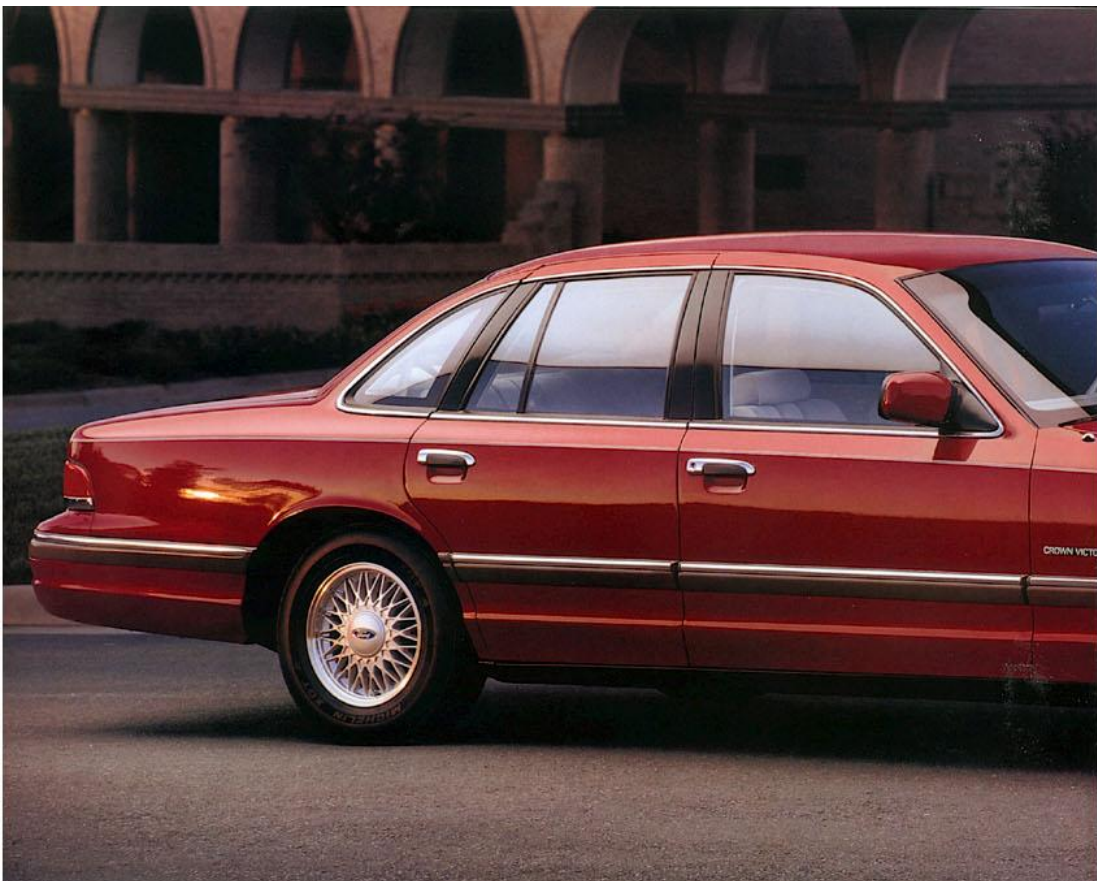
Crown Victoria's flush glass helps reduce noise caused by air turbulence. For convenience, the rear windows roll completely down.
