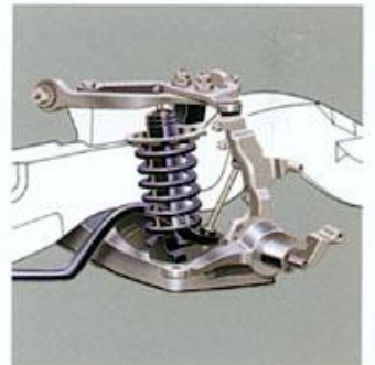
Adjustment cams on the front suspension's upper control arms allow precise wheel alignment for better handling and more even tire wear.
